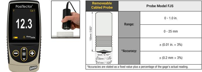
*FJS* - Removable FJS probe for measuring thick protective coatings on ferrous metal substrates. Ideal for thick epoxy, rubber, intumescent fireproofing and more.
