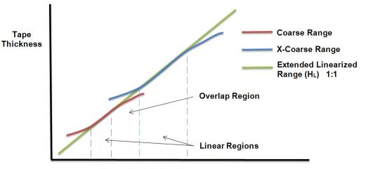
Figure 1 illustrates, schematically, the response function for each grade of tape. The blue curve (X-Coarse grade) shows, at the high end of its range, how the tape method reads low where peaks are higher than the foam' thickness, and, at the low end of the range, how tape reads high as it nears full compression. In between, X-Coarse exhibits a relatively linear response
