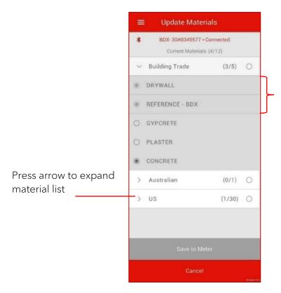
Greyed materials cannot be removed from meter (Drywall, Reference, and Douglas Fir)
