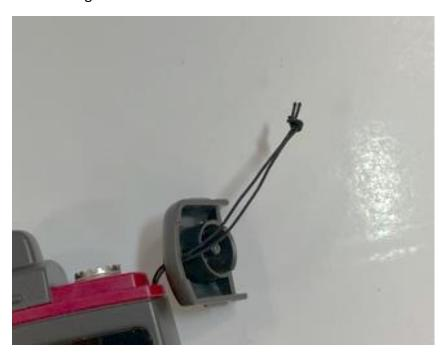
Step 5 – Slide the connector cap to the end so that the knot is inside and place the cap back onto the meter as shown.
