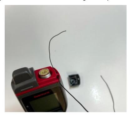
Step 3 – Feed both ends through the top side of the connector cap.
