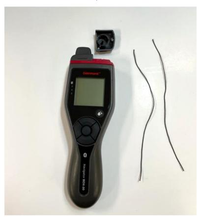
Step 2 – Thread one end of the Tether through the cavity of the meter.
