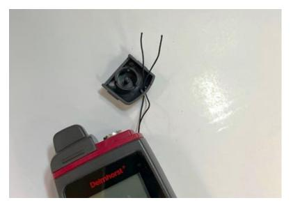
Step 4 – Tie a single knot on the end of the Tether.
