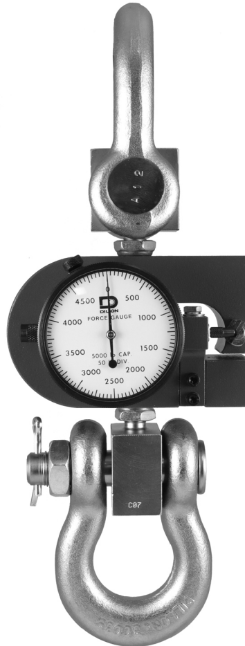
Figure 2.3 Tensile model with adapters and shackles
