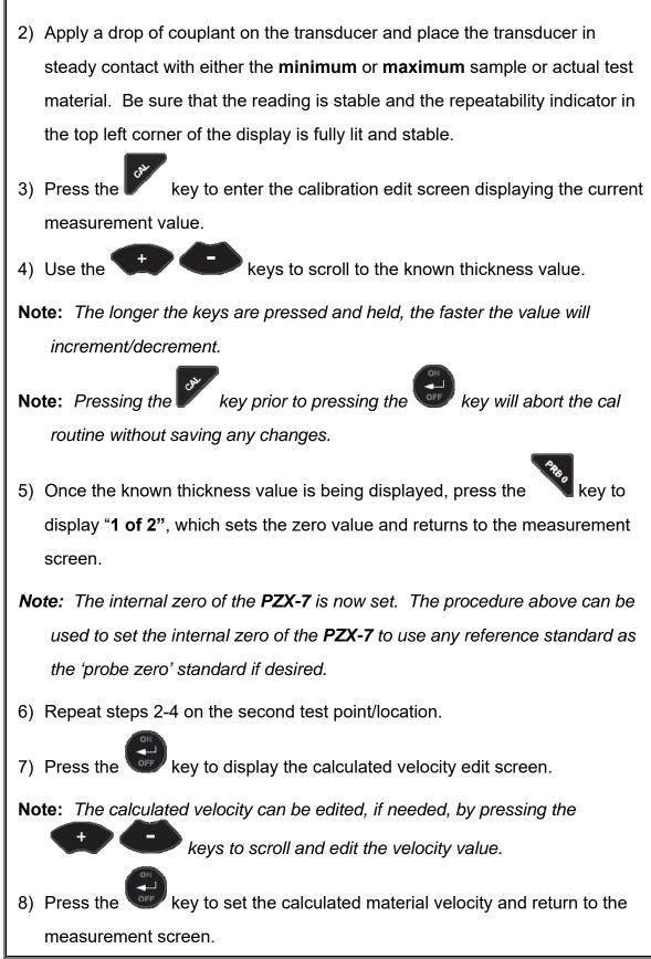
Note: CHECK YOUR CALIBRATION! Place the transducer back on the
