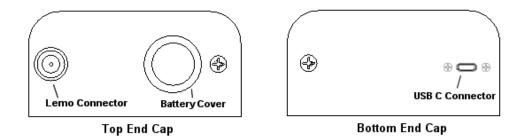
The top end cap is where all connections are made to the **PZX-7**. The diagram above shows the layout and description of the connectors:
