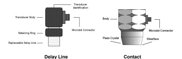
The Transducer is the "business end" of the *PZX-7*. It transmits and receives ultrasonic sound waves that the *PZX-7* uses to calculate the thickness of the material being measured. The transducer connects to the *PZX-7* using a single shielded coaxial cable with microdot connectors.
