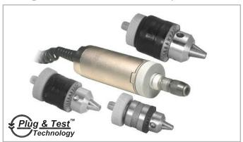
Series R51 smart sensors measure bi-directional torque for numerous applications across virtually all industries. Interchangeable Jacobs chucks and bit holder add flexibility for a variety of applications. The sensors can be used as hand held devices or mounted to a test stand. Superb overload protection adds peace of mind. Capacities available from 10 ozFin to 100 lbFin [7 to 1150 Ncm]. Compatible with Mark-10 model 5i and 3i indicators (sold separately) through unique Plug & Test™ technology.
