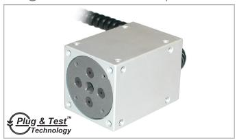
Series R52 smart sensors measure bi-directional torque for a wide variety of applications across virtually all industries. Calibrate torque tools, or use these sensors as components of a torque testing system. Tapped holes on every surface allow for easy mounting to a work bench or fixture. Capacities available from 10 ozFin to 100 lbFin [7 to 1150 Ncm]. Compatible with Mark-10 model 5i and 3i indicators (sold separately) through unique Plug & Test™ technology.
