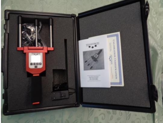
Figure 2: Carrying case with instrument, calibration certificate, charger, adapters, and operating instructions.
