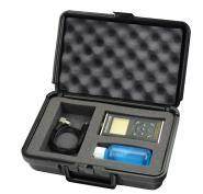
**Complete Kiti includes:** TI-25MX gauge, probe, 4 oz. bottle of coupling fluid, 2 AA batteries, NIST-traceable calibration certificate and operating instruction manual—all in a foam-fitted carrying case.
