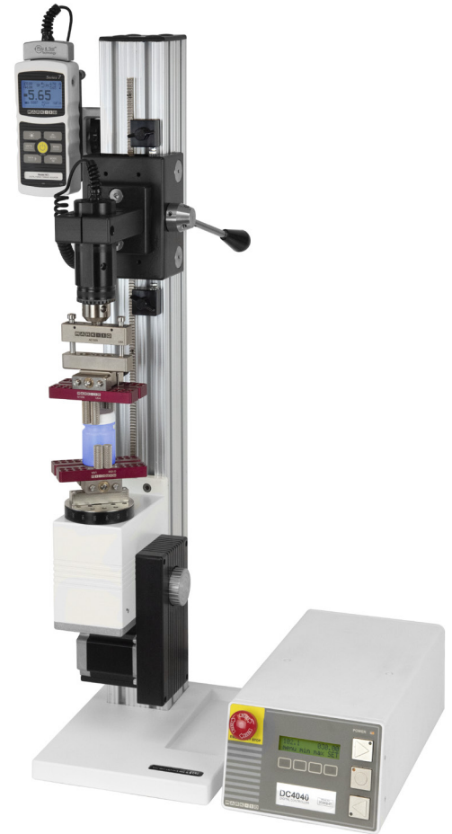
^ Model TSTM-DC is shown in a cap torque test, with a Series R50 torque sensor, M5i force/torque indicator, G1023 universal closure grip, and G1053 cap grip
