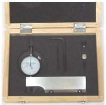
The Reaching Pit Gauge offers the equipment inspector many advantages over our Basic Pit Gauges (N88-2 or N88-3), with its Dial Indicator mounted at the end of the 152mm (6") long Blade, that features a long Cut-Away Nose.
