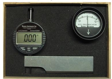
The Reaching Pit Gauge has been selected because Yellov Jacket (and other coatings typically end far enough back fron the weld that the coatings don' interfere with the Reaching Blade sitting flat on the Pipe surface The cutaway nose, on the dia indicator end of blade, permits positioning the Dial or Digita Indicator's Contact Point on eithe side of the weld.
