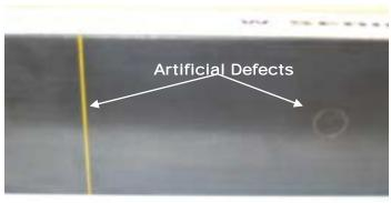
The Transverse Notch is approximately 0.016" Wide x 0.032" Deep (0.41mm x 0.81mm), is Epoxy filled, and extends the width of the Bar The Notch is positioned 2 ½" (63.5mm) from the one end of the bar, to allow either indication to be used.
